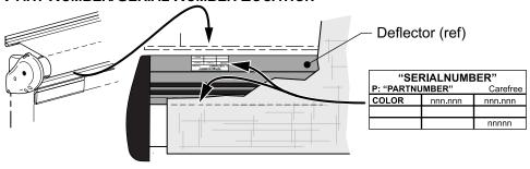
Serial Number/Part Number is located on the deflector beneath the canopy and on the roller tube
